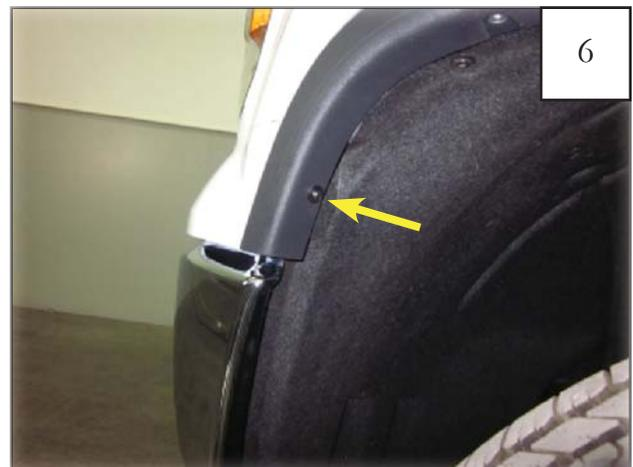
Remove fastener from front of factory wheel arch molding using a 9/32" or 7mm socket and wrench. Save for reinstallation.
